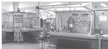
Just one example of the numerous filter testing procedures: Multipass test rig.
